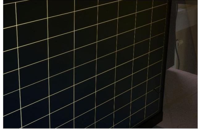
8. In the field, most likely the lower corners will diverge a bit, this is due to varying quality and manufacturing tolerances of the TFT panel fronts and mirrors (thickness and uniformity, resulting in different curvature), so in practice you'll see a picture like this, which is perfectly well within tolerance values:
