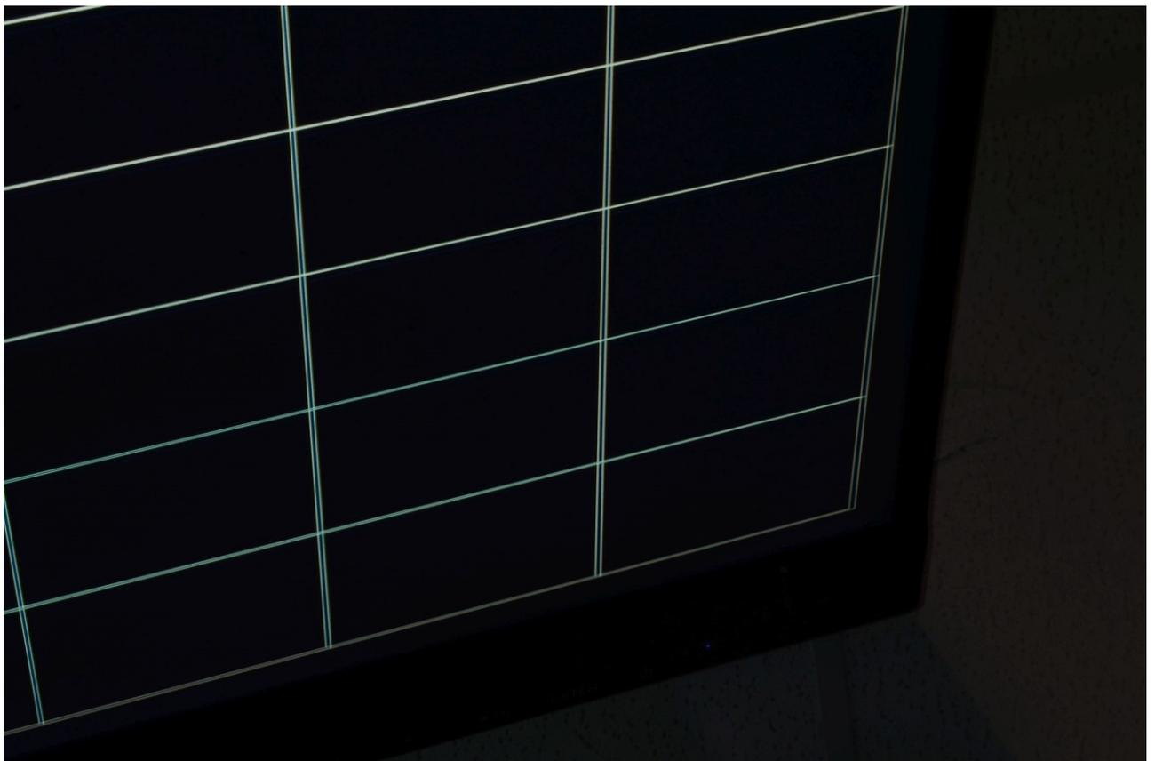
This slight distortion is only visible when viewing 2D content, like the test grid, without 3D glasses, which is not the field of application of the 3D PluraView – when viewing 3D content, the human eye perfectly compensates for this tiny drifts.
